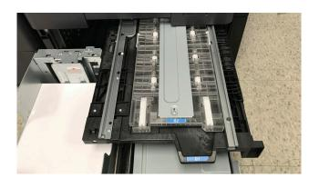
Misfeed areas are easily identified inside the machine with blue labels and numbers.
