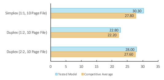
Single-set copy speed is tested using 3-page and 10-page mixed-color and black documents. Timing begins as the start button is pressed, pages are scanned through the document feeder and timing ends when the last page of a single-set of the document exits the device.
