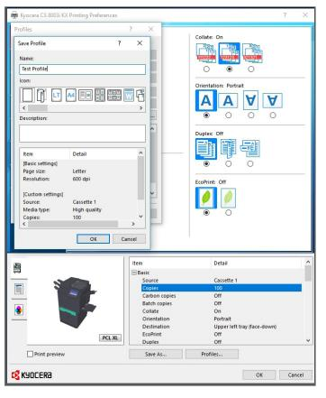
While an entire tab of the driver cannot be customized, users can save custom profiles that are stored as graphical icons via the Quick Print tab to allow programming of complex jobs in one click. Users can click on the Save As button on any of the tabs to save currently selected settings, name the new profile, and add a description for storage on the Quick Print tab. The order of custom profiles can also be prioritized.
