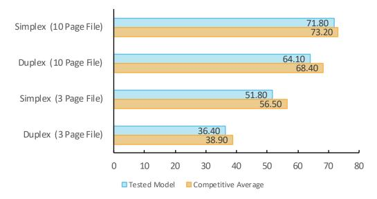
Speed is tested using Buyers Lab's proprietary 3-page and 10-page testing documents. Buyers Lab obtains the overall speed by averaging the tested speed for each run length (1, 5, 10, and 20 sets). The unit was tested using the PCL driver.
