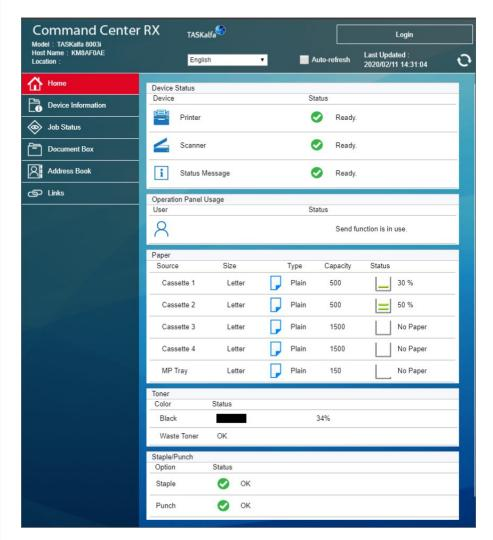
The main screen of the web user interface, Command Center RX, includes notifications and gauges on the status of the device including device state, and paper drawers and consumables in percent increments. Print, scan, and copy usage can be restricted and tracked by user and group. Up to three event reports can be set up and scheduled for when to add paper, add toner, cover open, paper jam, low toner, waste toner replacement, and other errors.
