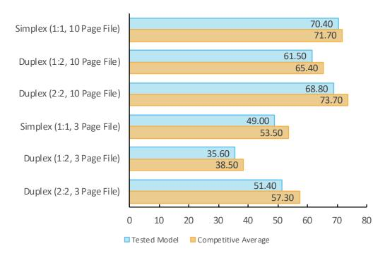
Copy speed is tested using 3-page and 10-page mixed-color and black documents. Buyers Lab obtains the overall speed by averaging the tested speed for each run length (1, 5, 10, and 20 sets).
