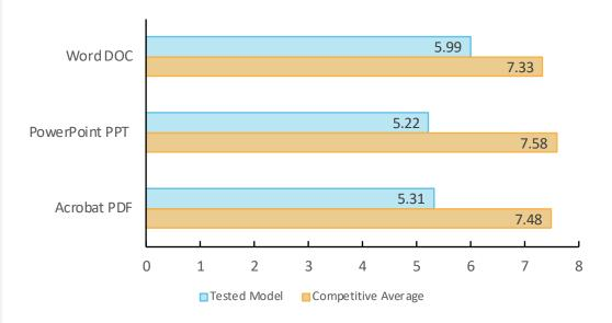
First-print time indicates the time it took to process the image and deliver a single-page test document to the output tray. The unit was tested using the PCL driver.
